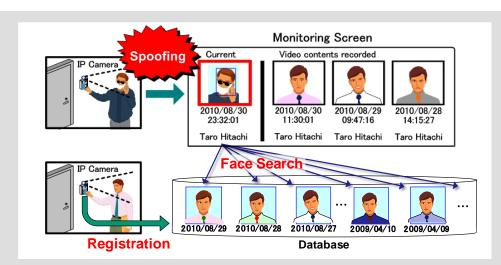
Hitachi, Ltd. and Hitachi Information & Communication Engineering, Ltd., have developed masquerade detection technology for IC card access control systems based on face recognition of images recorded on each entry/exit.
